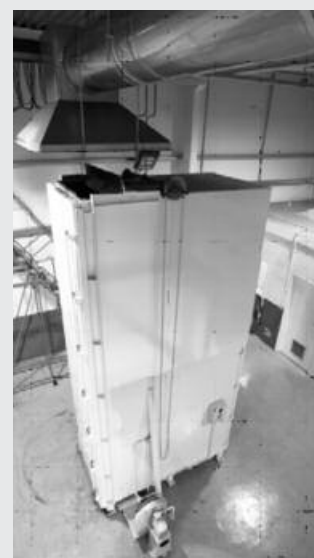
Example of CPD test chamber acc.to prEN50399
